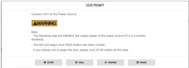
The test progress is communicated to the operator in real time and allows for pausing or aborting at any time if desired.
