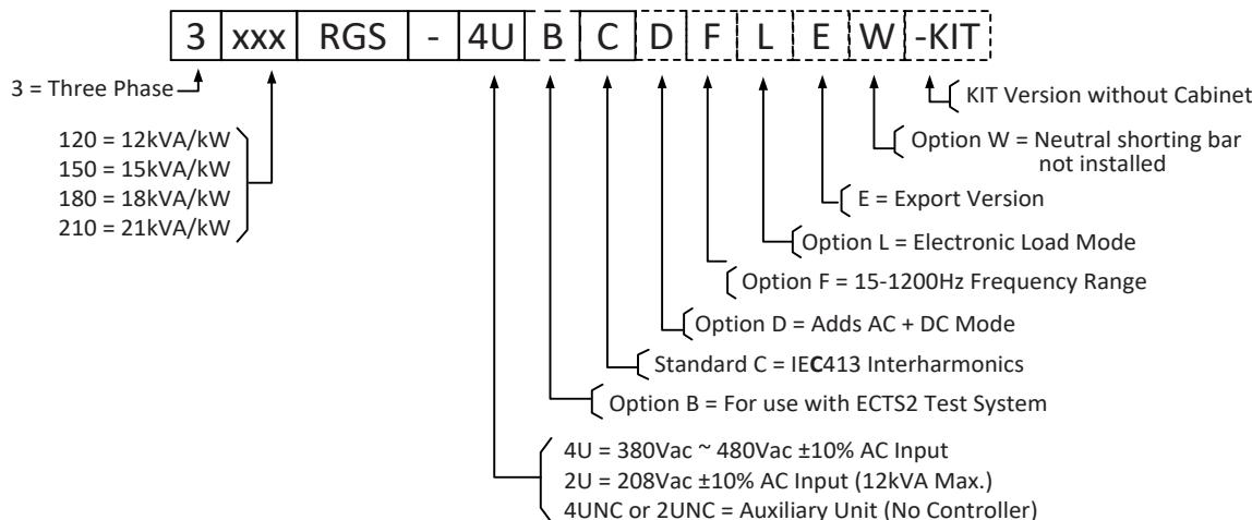
NOTE: 4U indicates that the shorting bar for output neutrals will be installed on the units by default. If Option W is selected, the units will be shipped with shorting bar for neutrals removed and provided in the ship kit instead.
