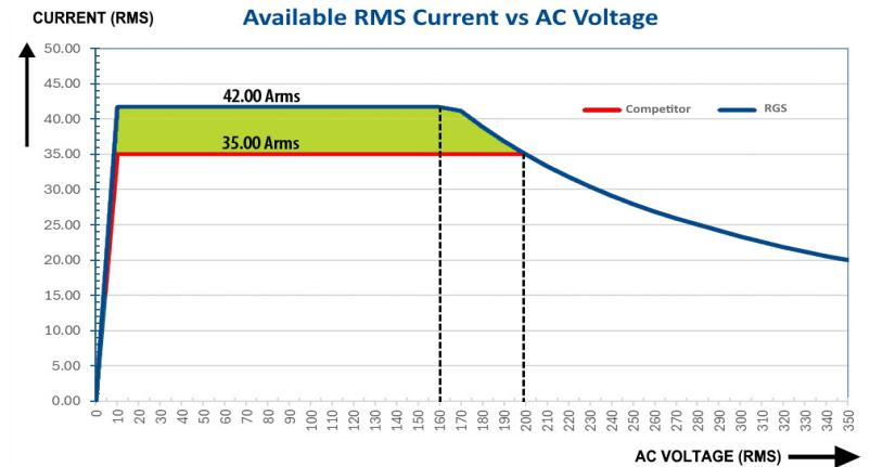
The RGS provides 20% more current from 120V to 200V compared to a typical unit that maxes out at 35A/phase.
