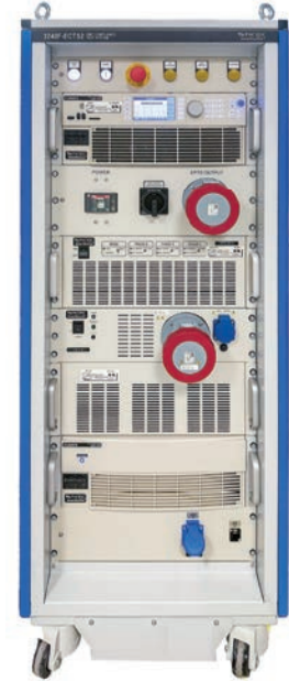
ECTS2 EMC Test System with integrated EPTS-3-100A Voltage Dips Module
