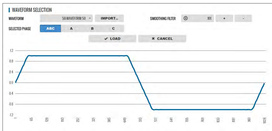
Figure 6-9: Same Waveform with maximum smoothing Filter Applied
