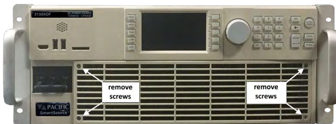
Figure 5-7: Air Intake Filter Removal
