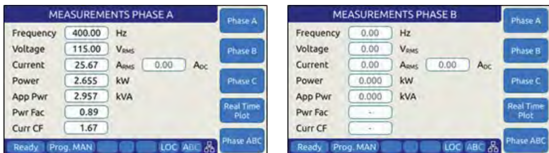
Figure 6-7: Single Phase Measurement Screens for Phase A and B
