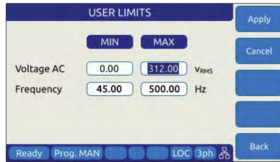
Figure 6-5: Enable Vac extended operating range to 312Vac
