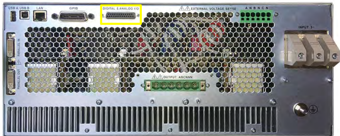
Figure 7-1: Rear Panel AUX I/O DB25 Connector Location
