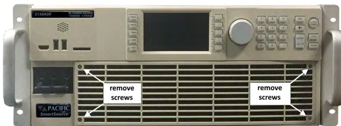
Figure 5-7: Air Intake Filter Removal
