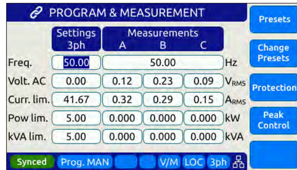
Figure 7-4: External Sync Input Sync Status Indication
