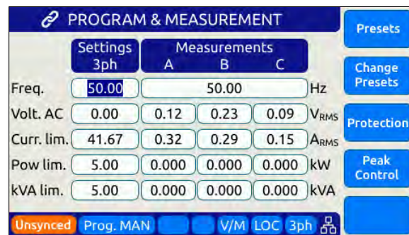
Figure 7-5: External Sync Input Sync Lost Status Indication
