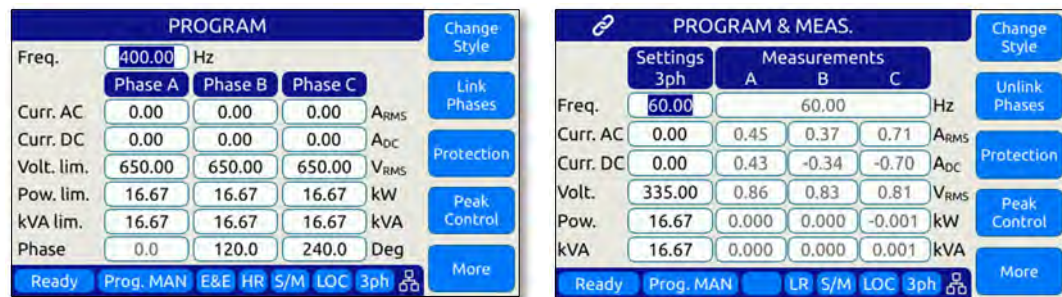
Figure 6-3: PROGRAM Screens Current Source Mode
