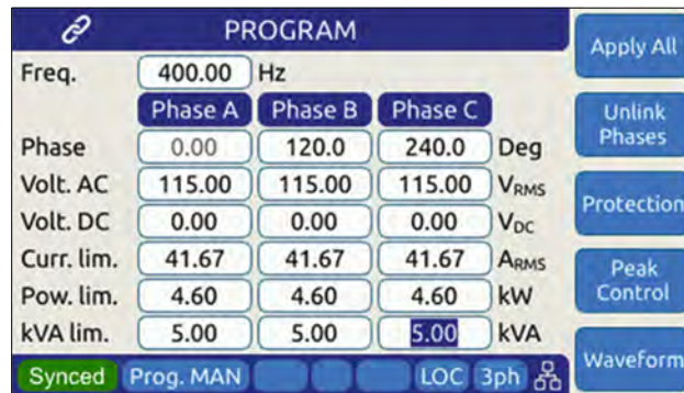
Figure 7-4: External Sync Input Sync Status Indication
