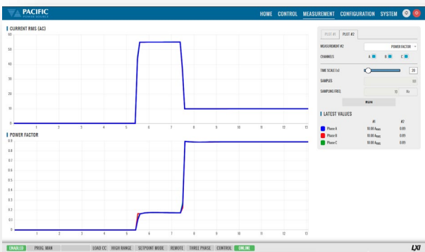
Test of motor drive running for 2s at 55A at .02 PF (inductive)
