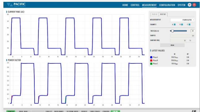
This diagram illustrates the condition of starting, stopping, then restarting the motor repeatedly.
