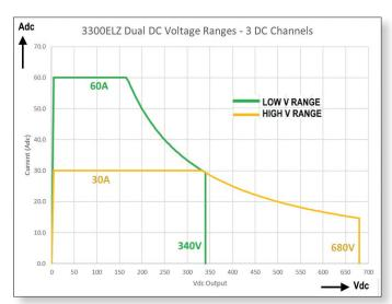
Figure 4: High and Low DC Voltage Ranges - Current vs. Voltage - 30kW
