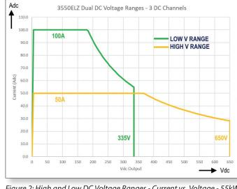
Figure 2: High and Low DC Voltage Ranges - Current vs. Voltage - 55kW
