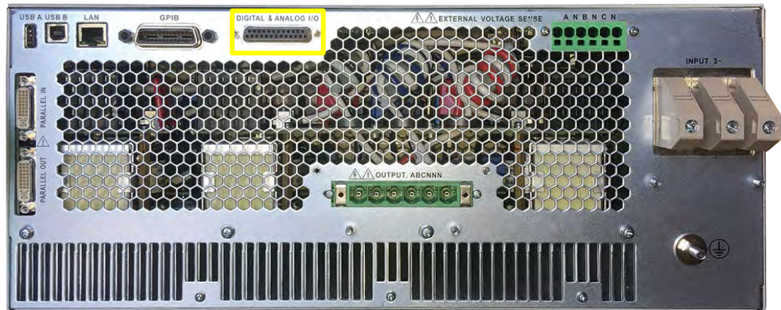
Figure 7-1: Rear Panel AUX I/O DB25 Connector Location
