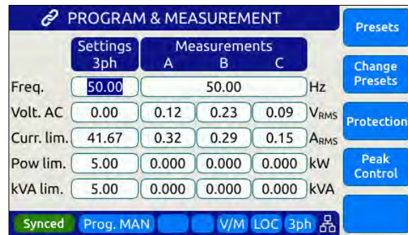
Figure 7-5: External Sync Input Sync Status Indication
