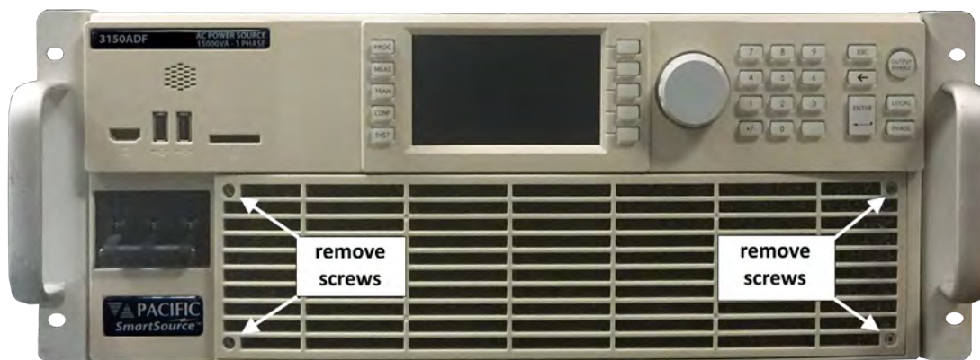
Figure 5-6: Air Intake Filter Removal
