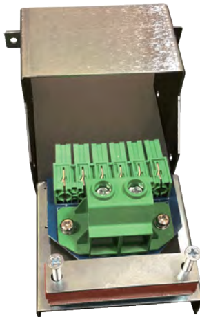
Figure 5-12: 1150ADF or 3150ADF-M Single Phase Shorting Adaptor assembly
