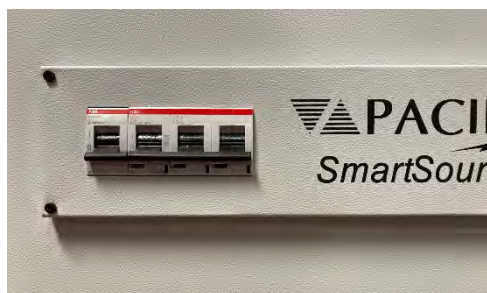
Figure 5-3: Mains CB in OFF (lower) Position
