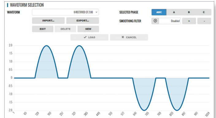
Figure 11: Three Phase AC Rectifier Current Waveform
