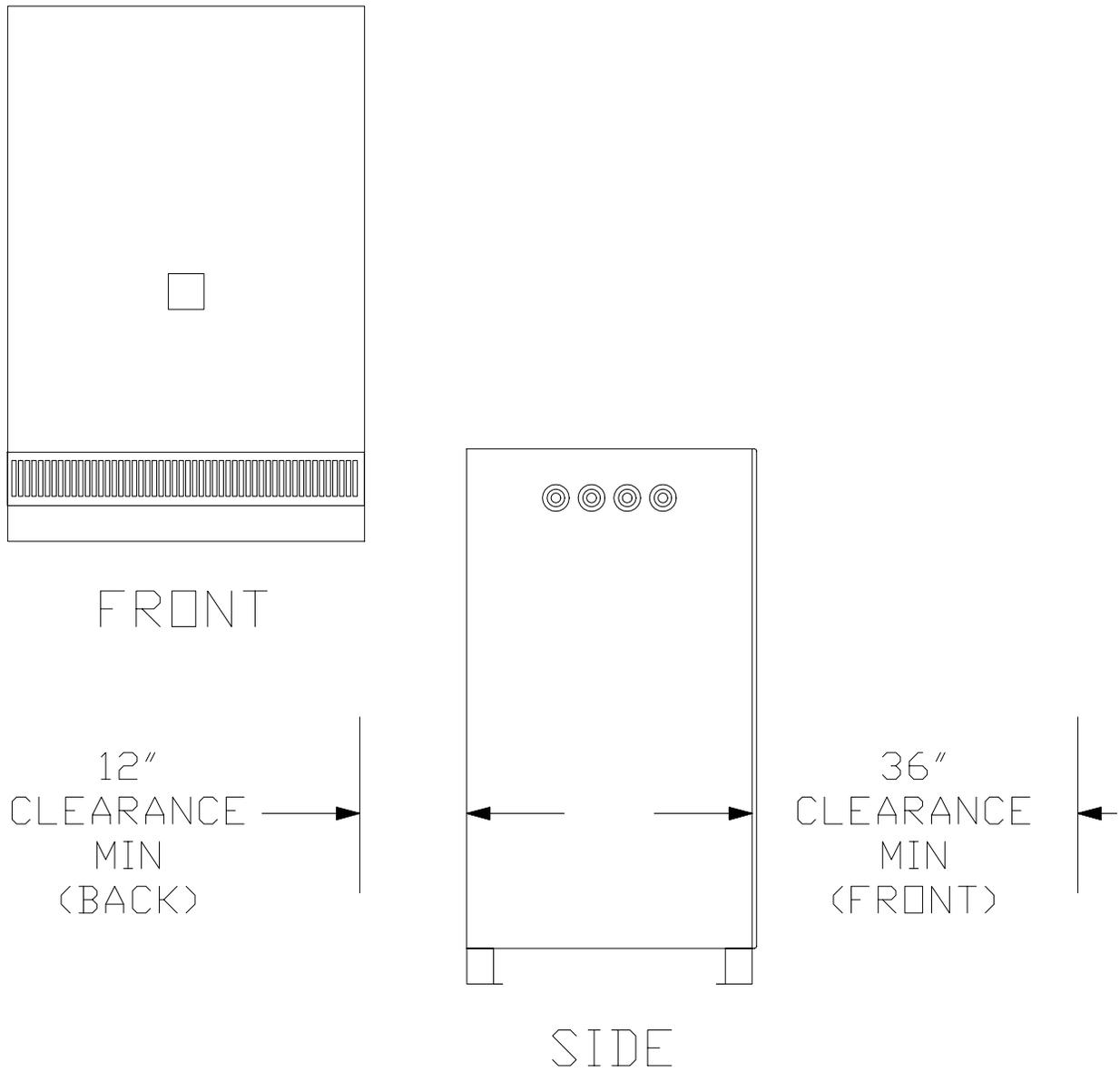
**FIGURE 3.7.1 BATTERY CABINET SERVICE CLEARANCES**
