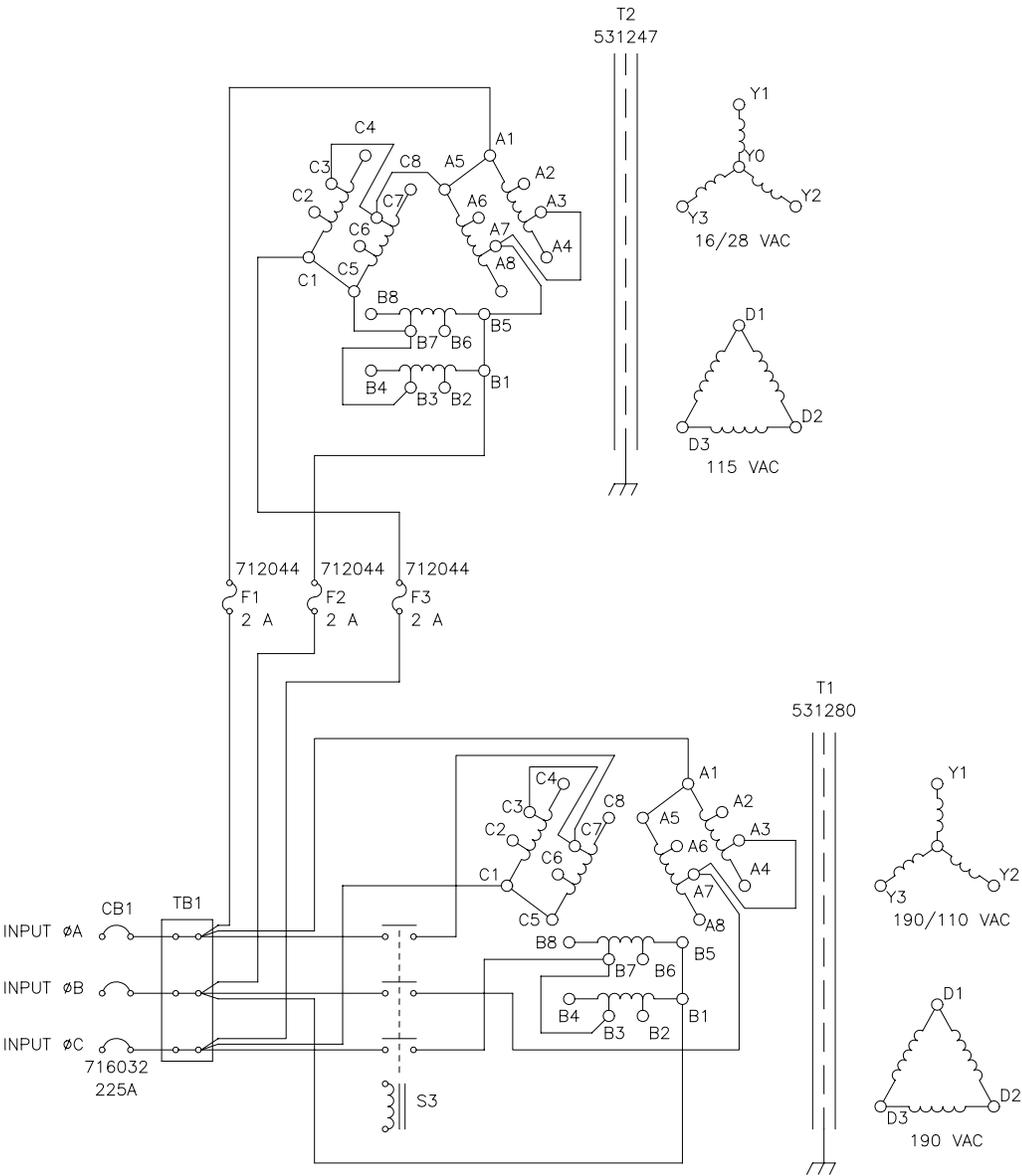
**FIGURE 3.3.4 208 V INPUT CONFIGURATION**
