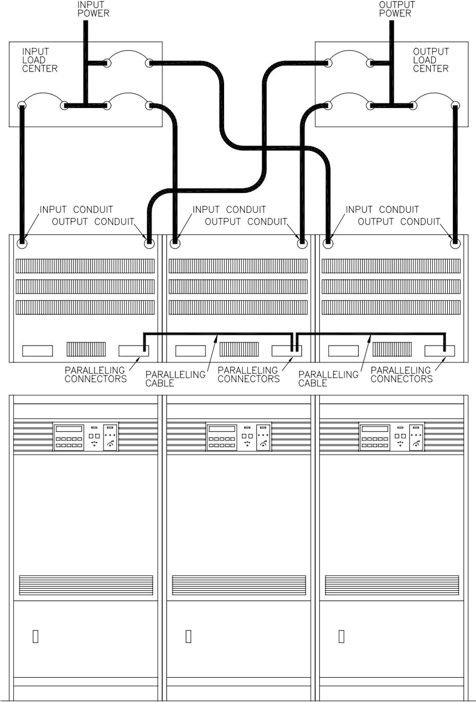
FIGURE 3.8.2 MULTIPLE CABINET SYSTEM ONE-LINE DIAGRAM
