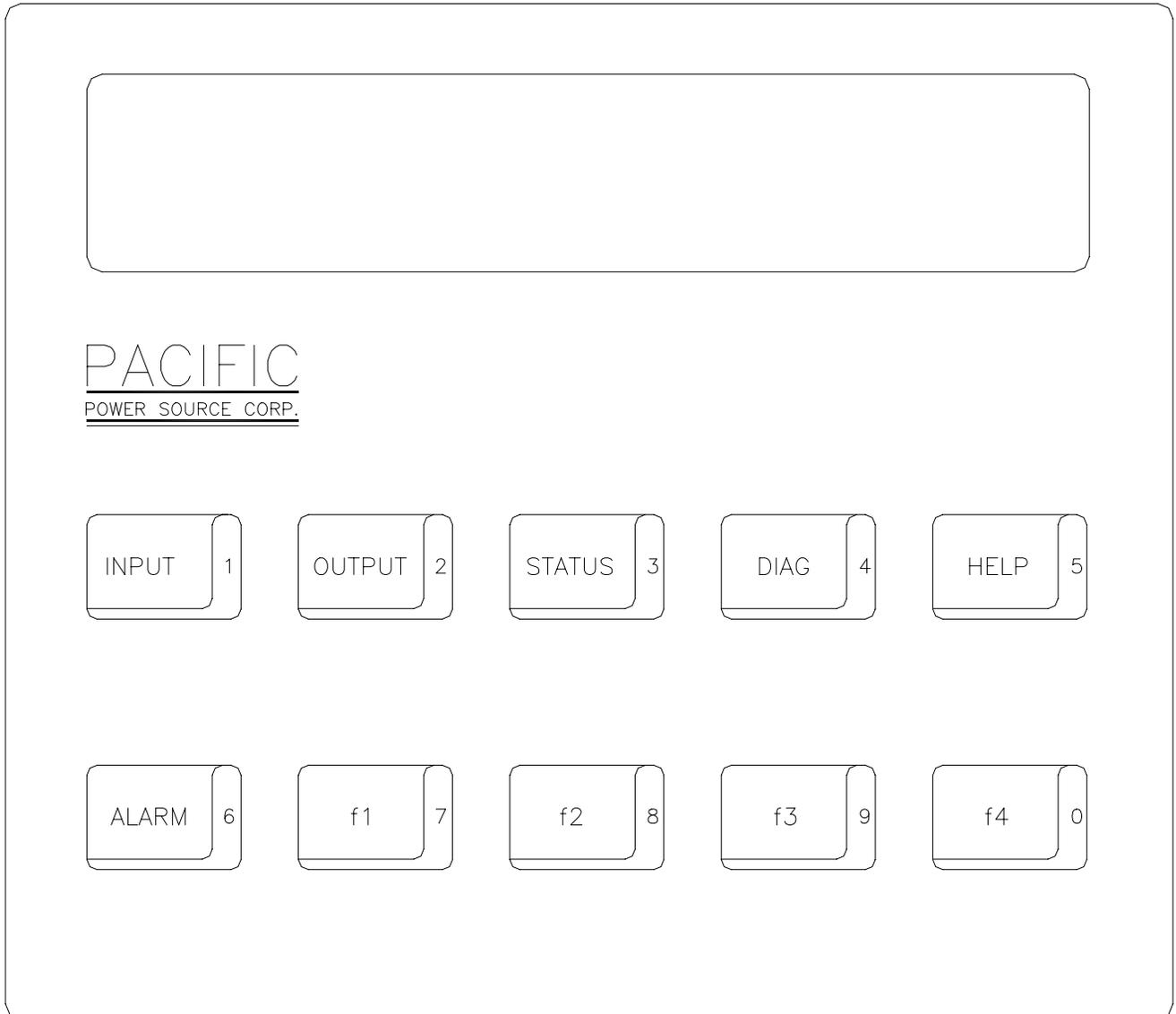
FIGURE 4.4.1 LCD AND INTERROGATION SWITCHES
