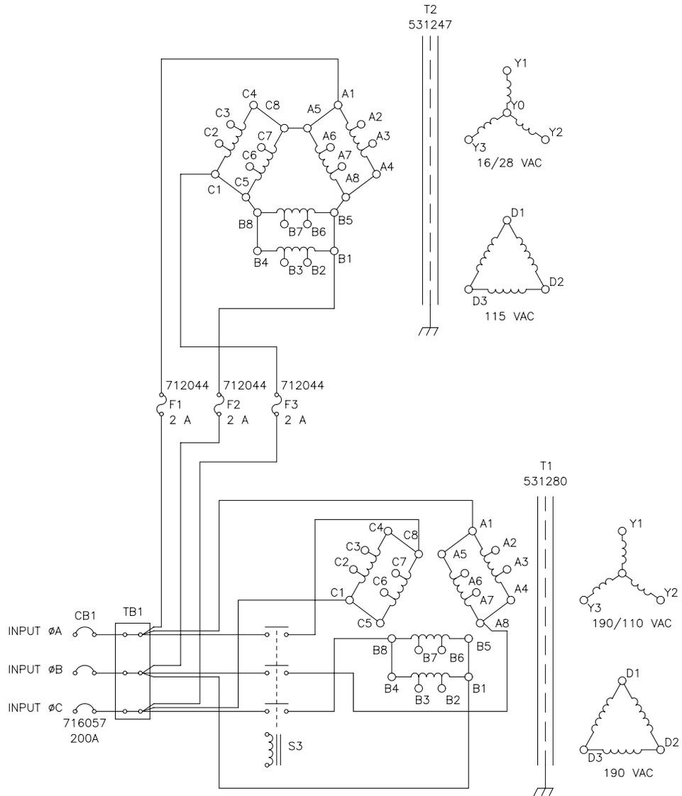
**FIGURE 3.3.3 240 V INPUT CONFIGURATION**
