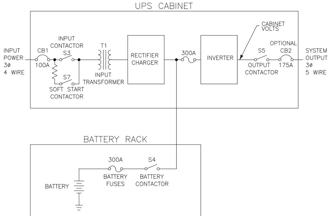
**FIGURE 1.3 UPS FUNCTIONAL BLOCK DIAGRAM**
