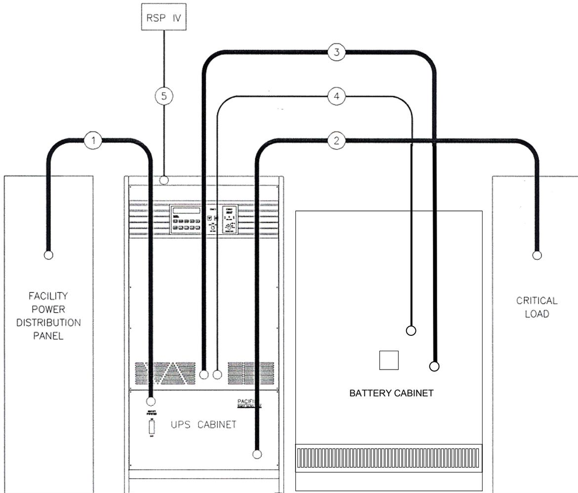
FIGURE 3.4A SYSTEM INTERCONNECT WIRING
