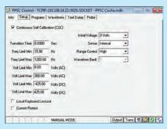
Configure Output Modes, User Limits and Self Calibration mode from the PPSC Control screen.
