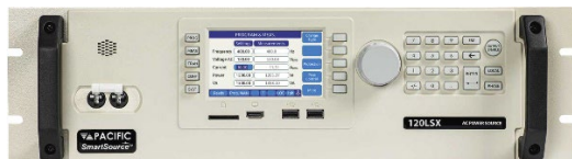
Model 120LSX single phase, 2kVA AC Source for small HVAC units.
