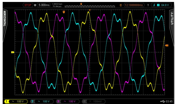
Figure 2: IEC 61000-4-13 Inter Harmonic Frequency Sweep Test
