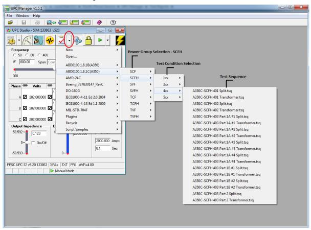
ABD0100.1.8.1C-A350 test sequences are grouped based on categories of equipment defined in the test standard: SCF, TCF, SVF and TVF. The individual test sequence files are named using the following naming convention:
