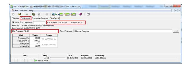
If a test engineer will be modifying a test sequence, it is recommended that a copy of the original file first be saved in a different folder as changes overwrite the existing file. For detail information on test sequence modification, please see UPC Test Manager Operation Manual.
