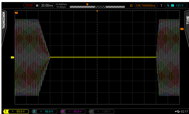
Figure 14: DO-160G Section 16.5.1.4 b Test Condition 7
