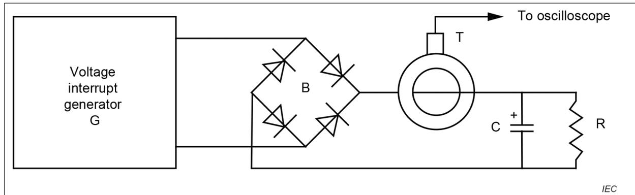
Figure 3: Test Setup to verify AC Power Source Peak Inrush capability
