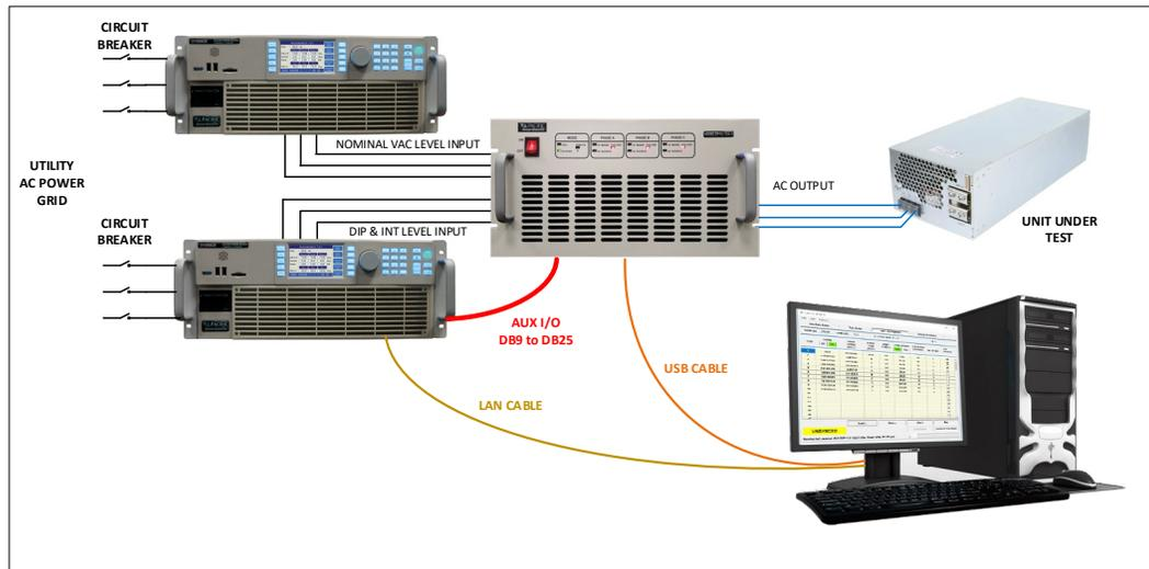
Figure 2: Dual AC Source EPTS— Test Setup
