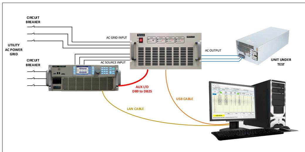
Figure 1: Standard EPTS Test Setup
