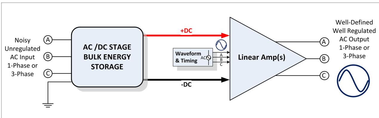
Fig. 2. AC to AC Linear Amplification Power Conversion
