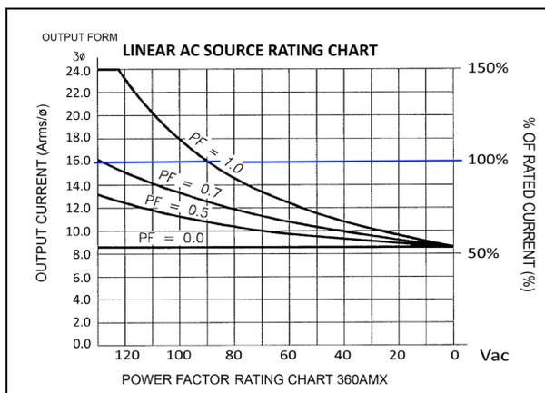
Fig. 4. Linear AC Source Rating Chart
