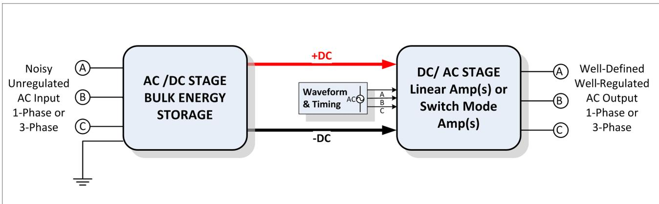
Fig. 1. Fundamental AC-to-AC Power Conversion
